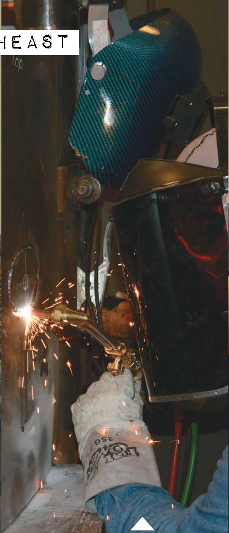
MAX SMITH, L-154 , uses an Oxy-Acetylene torch to cut out an elliptical penetration for a nozzle on a rolled tank sheet.
