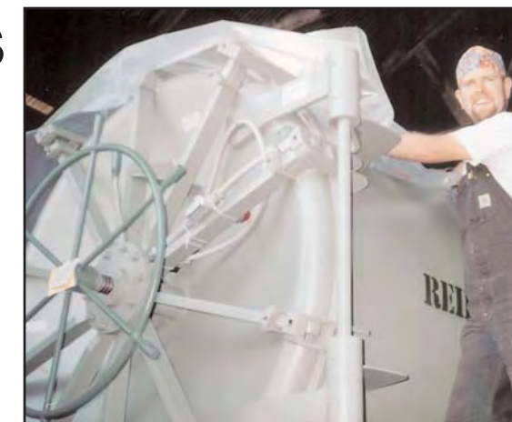
Marty Scott adds the final touches to a retort (pressure vessel sterilizer) at Reid Boiler Works.
