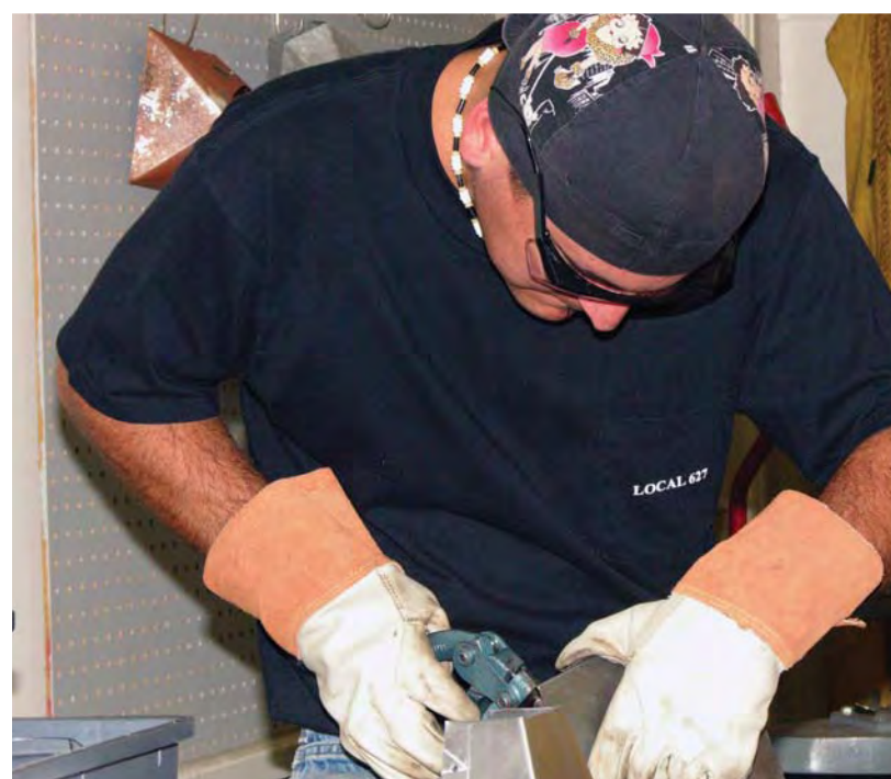
Jayme Taylor (L-242) does light riveting in the metal fabrication test.
